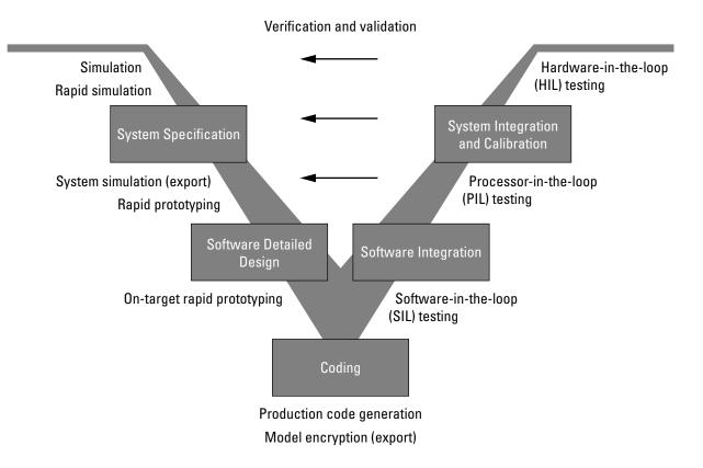
Depending on your application and role in the process, you might focus on one or more of the steps called out in the V or repeat steps at several stages of the V. Real-Time Workshop technology and related products provide tooling you can apply at each step.
