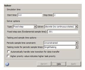
For Real-Time Workshop software to generate code for a model, you must configure the model to use a fixed-step solver. The start and stop time do not affect generated code.
