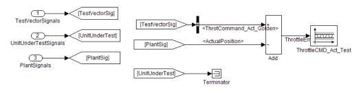
**5** Open the *plant or feedback system*, implemented in this test harness as the Plant subsystem.
