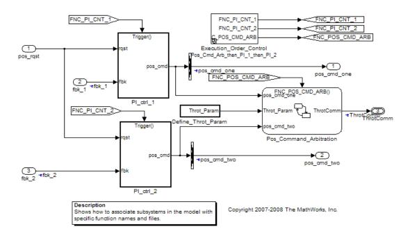
The Execution\_Order\_Control subsystem has been added to the model. It is a Stateflow chart that models the calling functionality of a scheduler. It
