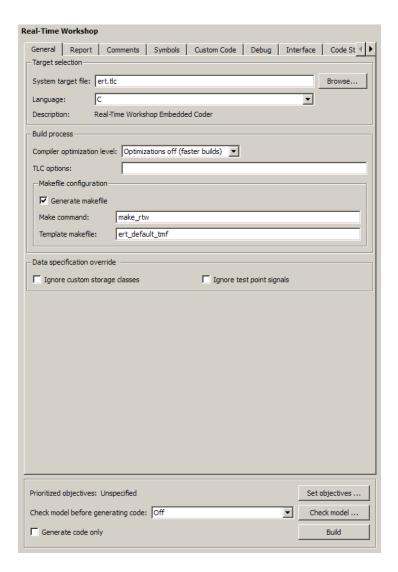
The **Real-Time Workshop** pane is where you specify the system target file (STF) and the language for your generated code. This demo model uses the Real-Time Workshop Embedded Coder STF (ert.tlc) and the C language. You can extend the STF to create a customized configuration. Some of the basic configuration options reachable from the **Real-Time Workshop** pane include:
