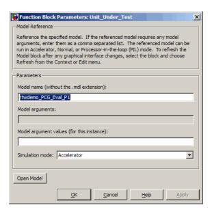
The Model block allows you to reference other models (directly or indirectly) from the top model as compiled functions. By default, Simulink software recompiles the model when the referenced models change. Compiled functions have several advantages over libraries:
