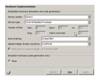
Use hardware implementation parameters to specify the word size and byte ordering of the target hardware. This demo model targets a generic 32-bit embedded processor.
