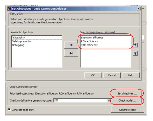
The Code Generation Advisor dynamically creates the list of checks based on the objectives that you select. The first check reviews the current values of the configuration parameters and recommends values based on the objectives. The check provides an automated method for setting the parameters to the recommended values.
